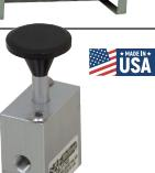
• New, SAF HOLLAND model XB-11745 fifth wheel release valve. Pull knob, spring return. For kingpin or slider lock release. Ports labeled on valve body as #1 Delivery Port, to the fifth wheel slide assembly, and #2 Supply Line, from the truck.
